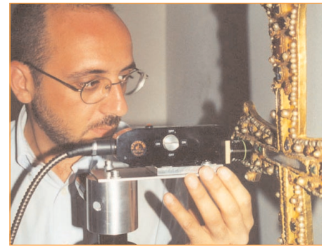
Using a RP10 compact probe and a manual tripod to analyse the gemstones in a gold cross.
