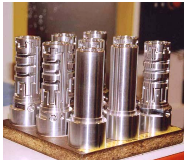
Machined spindles – tight tolerances and good surface finish is paramount
