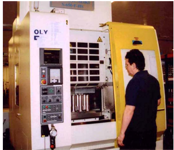
Machining centres, equipped with job set-up probes, can now run batches of multiple components
