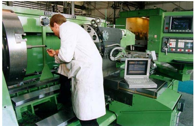
QC10 ballbar test on a Binns & Berry machine, cutting production time by an average of one day per machine
