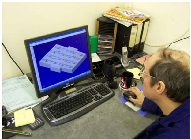
The process starts with a CAD model like this one for the Aquapac, which is used to create the machining program
