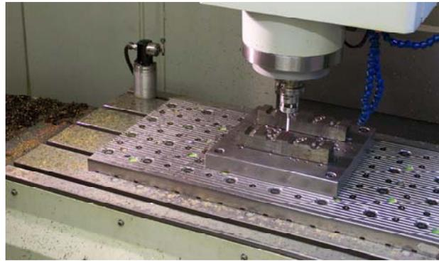
The spindle-mounted probe is used to set the Aquapac mould tool for roughing and semi-finishing operations
