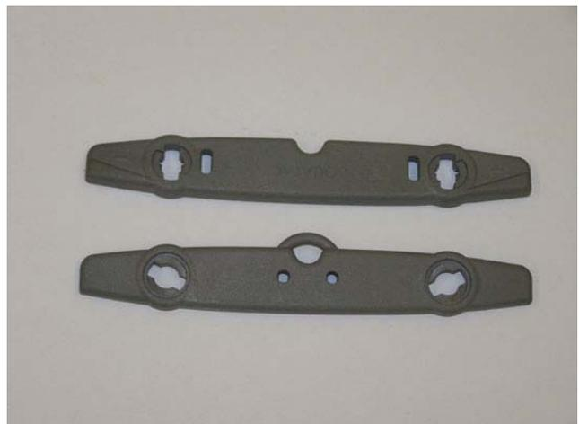
The finished Aquapac clamp comes straight from the injection moulding machine requiring no further finishing operations
