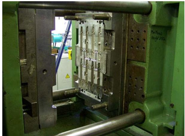
The finished multi-part tool is proven on BK Tooling's own injection moulding machine
