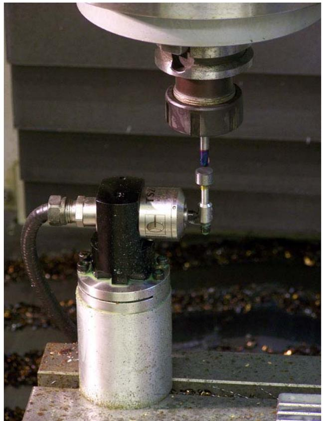
Tool setting on the machine is fast and takes into account thermal effects
