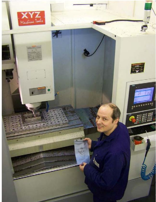
Bob Tunks with the XYZ HS 1060 high-speed machining centre - he relies on Renishaw touch probes for setting parts accurately, measuring them in-cycle, and for setting tool lengths
