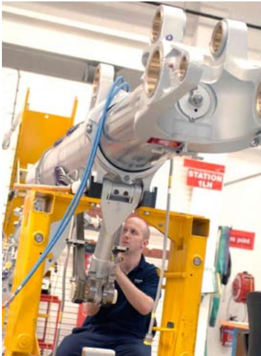
Landing gear for Airbus being assembled
