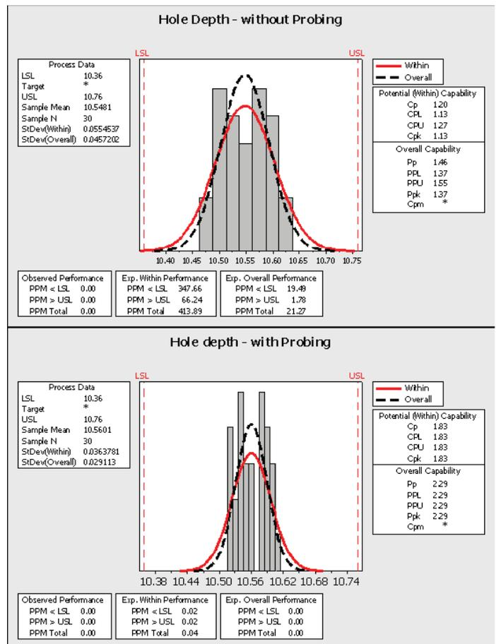
**Significant improvements in process capability resulting from automated in-process control.**
