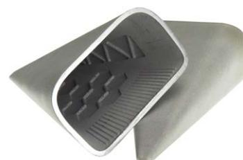
We believe that the key benefit of using an additive manufacturing process to produce the nose tip is the ability to create a hollow tip to minimise weight. To machine this component conventionally would be extremely challenging, result in design compromises, and waste as much as ninety five per cent of the expensive raw material.
