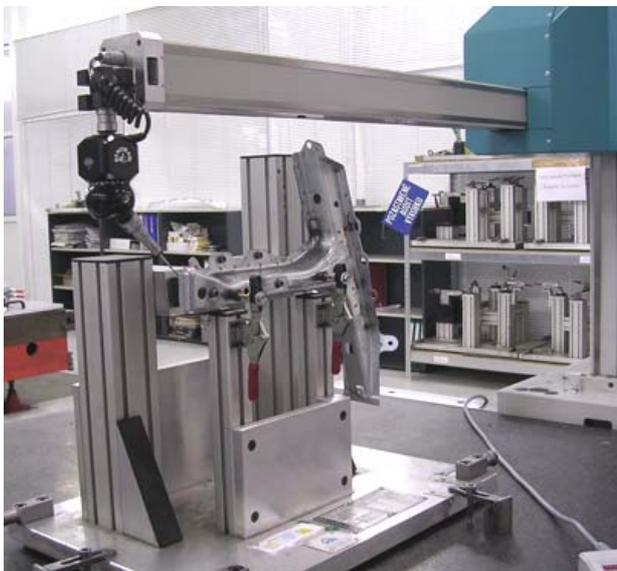
Computer controlled automatic CMM measuring sample welded assembly, accessing every feature in one set up
