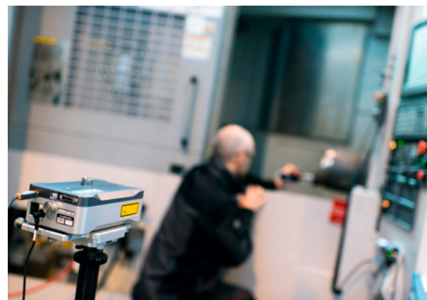
Craig Simpson, Maintenance Technician at FMC Technologies, using the XL-80 laser calibration system to check machine accuracy
