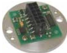
The layout of the pads on the board is suitable for the MOLEX 43045-1219 connector (mating part MOLEX 43025-1200 + crimp terminal 43030-xxxx).
