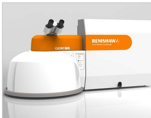
The Renishaw inVia Qontor confocal Raman microscope
