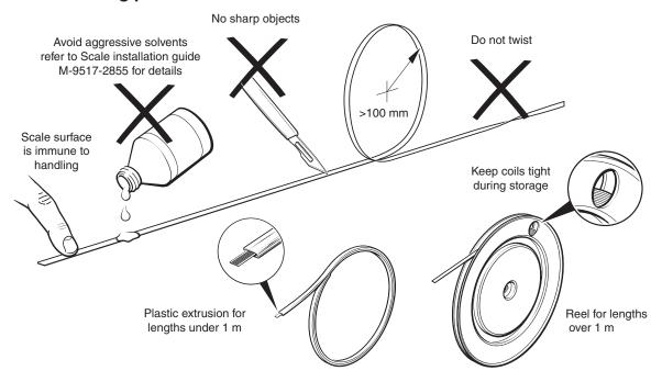
DO NOT remove the scale for refitting or use elsewhere once it has been applied to the mounting surface.
