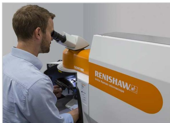
Renishaw inVia Qontor® confocal Raman microscope
