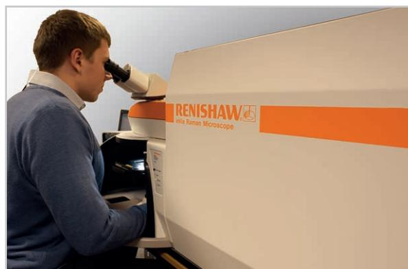
The Renishaw inVia confocal Raman microscope
