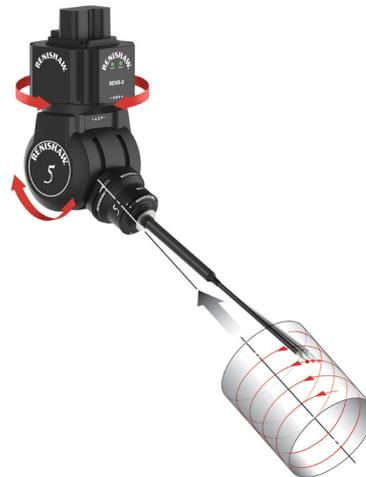
*In 5-axis measurement the CMM moves at a constant velocity whilst the REVO-2 head performs all rotation and modulates probe deflection, simultaneously controlling the three machine axes and the two head axes.*
