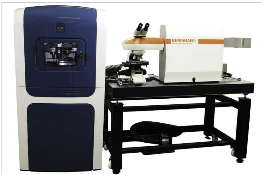
A TI 950 TribolIndenter (Hysitron, Minneapolis, Minnesota, USA, [www.hysitron.com](http://www.hysitron.com)) coupled to an inVia confocal Raman microscope via a separate fibre optic probe.
