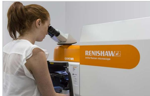
*The Renishaw inVia confocal Raman microscope.*
