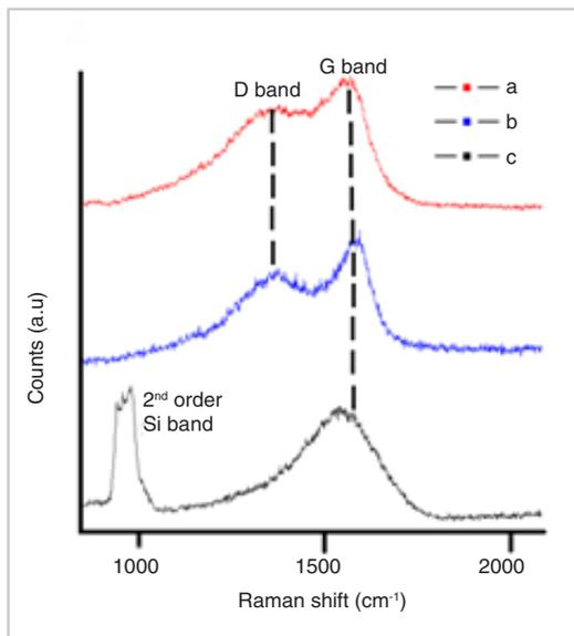
Figure 1. Raman spectra of DLC samples a, b and c.
