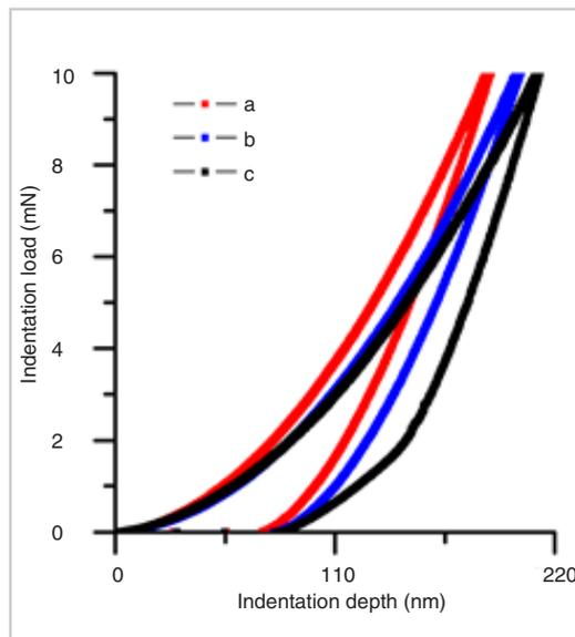
Figure 2. Indentation curves for samples a, b and c. A maximum normal force of 10 mN was used for each sample.
