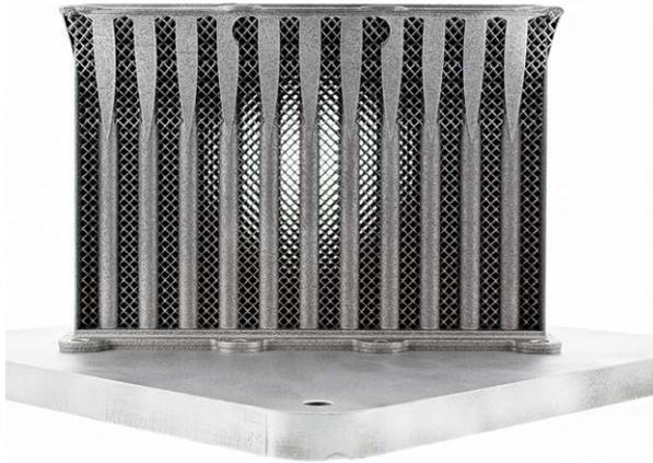
Intercooler on the build plate showing mesh detail
