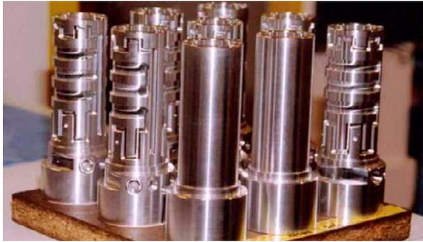
Machined spindles - tight tolerances and good surface finish is paramount
