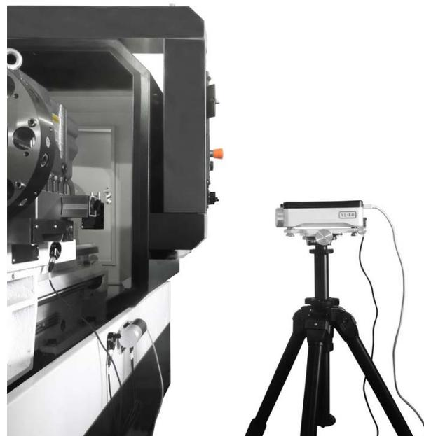
Checking accuracy of movements in machine tools with XL-80 laser system
