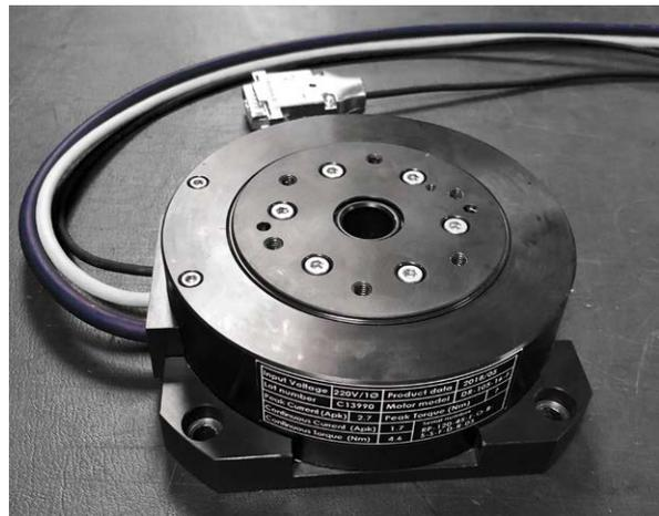
ATOM optical encoder in a mini rotary platform application
