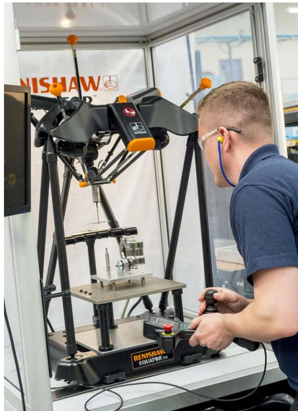
Equator system being used to inspect programmed aerospace part
