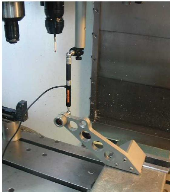
*QC10 ballbar checking X-Z positioning performance of one of TJW's HAAS machines. Spindle probes and non-contact tool setting systems transform setting time and consistency*
