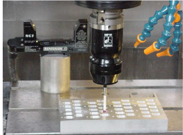
*Spindle probe setting a pharmaceutical part, non-contact tool setter in the background*
