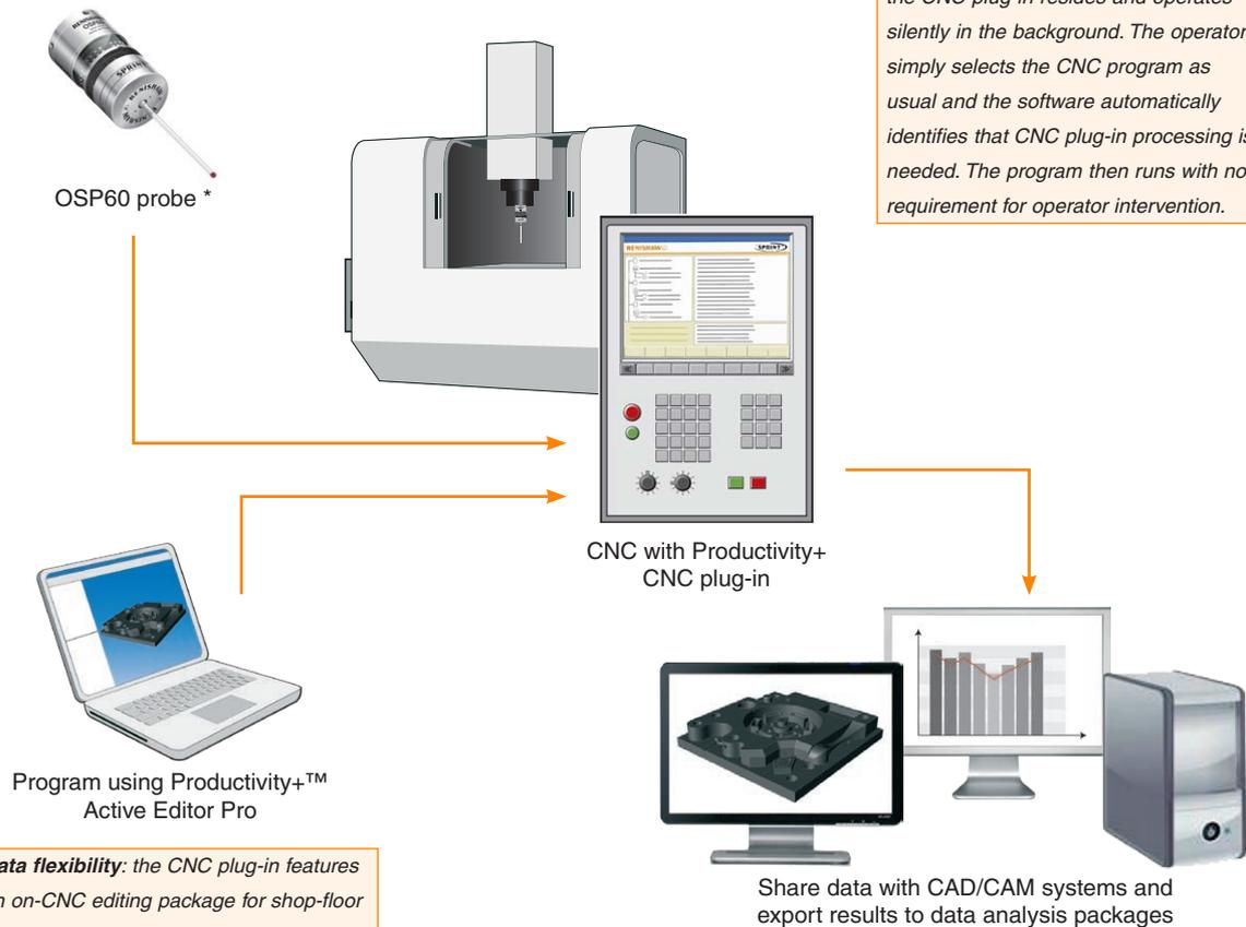
**Data flexibility:** the CNC plug-in features an on-CNC editing package for shop-floor program creation and editing. Programs can also be authored in a stand-alone editor, or in the CAM environment using a Productivity+ enabled system.
