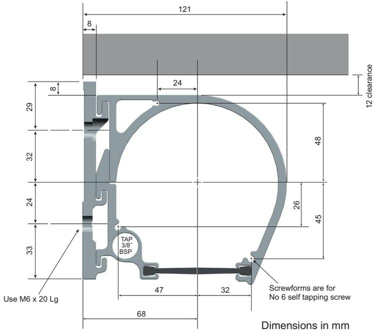
Figure 4 – Low profile ducting cross section
