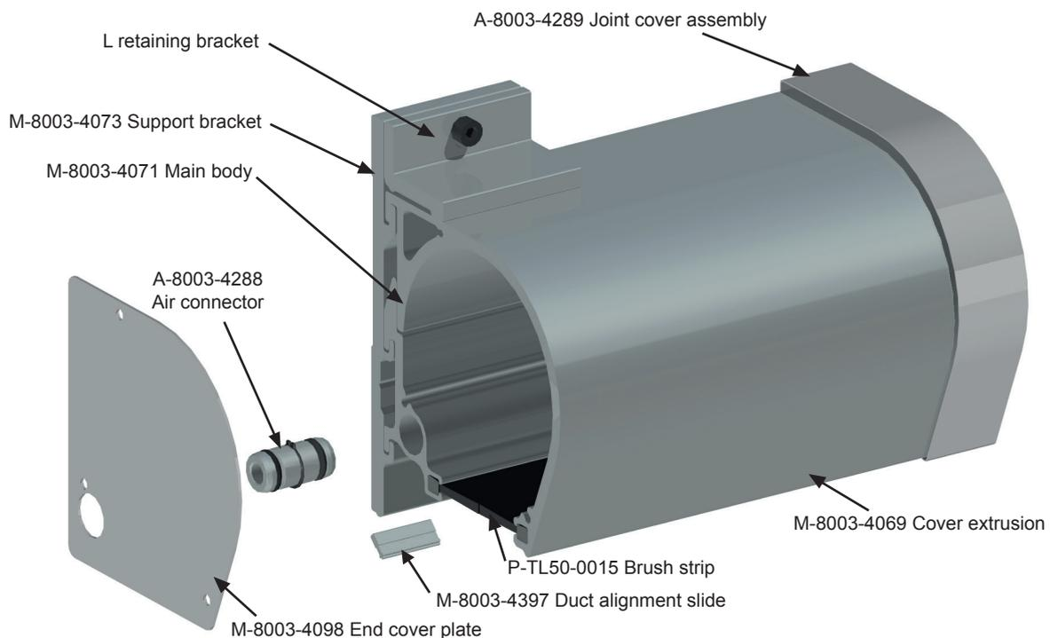
Figure 1 – Main parts assembly drawing (standard ducting)
