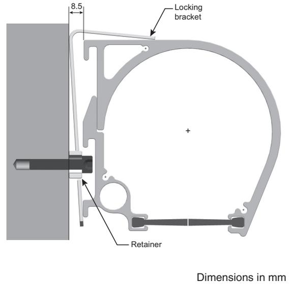
Figure 5 – Low profile ducting (view includes locking bracket)
