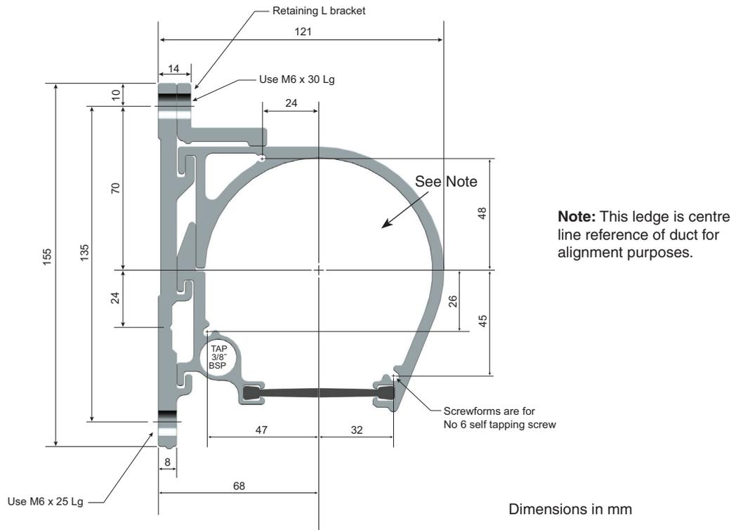
Figure 3 – Standard ducting cross section
