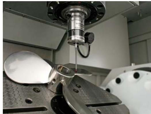
RMP600 high accuracy radio-transmission touch probe
